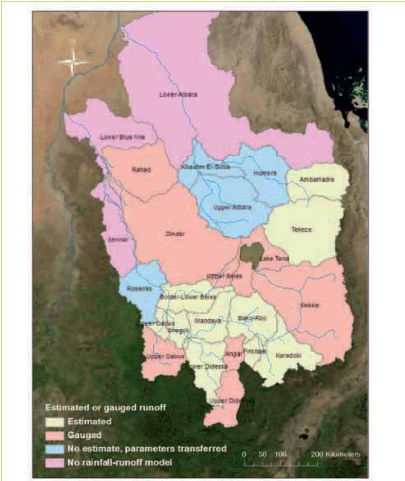
Figure 5.44 Approaches to estimating runoff for model calibration
