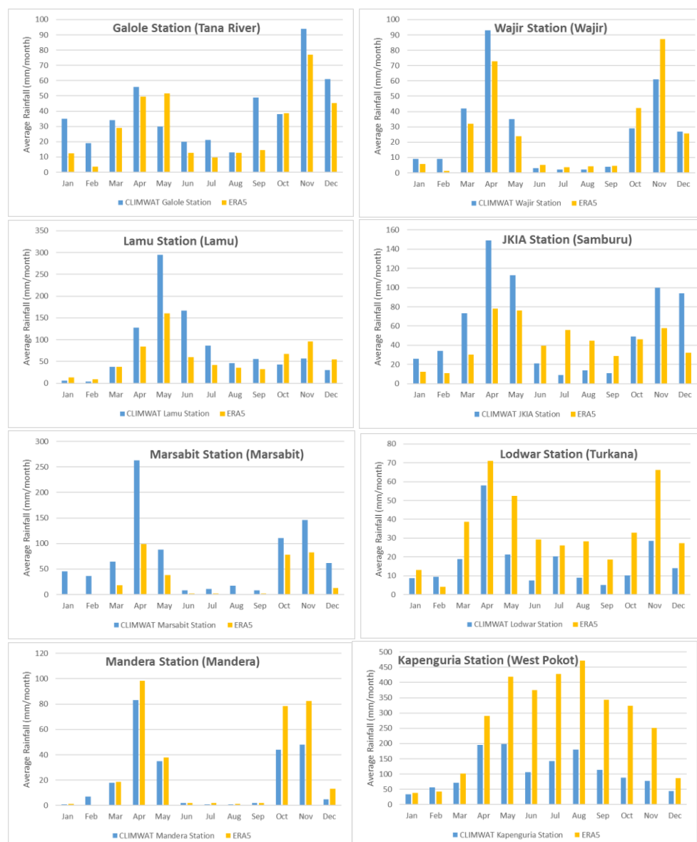
Figure 7-4 Comparison of CLIMWAT ground station rainfall data (for minimum 15 years within 1971 – 2000) and ERA5 rainfall (2003 – 2020) extracted at the point location of the ground station.
